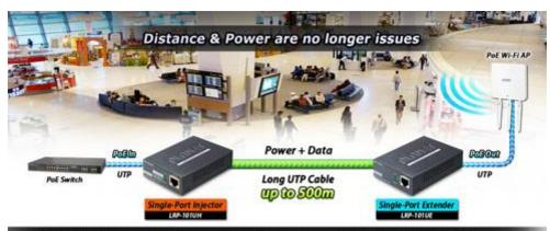
Extend IP Ethernet transmission and inject power beyond the 100 meters 1-Port Long Reach PoE over UTP Extender Kit (LRP-101UH + LRP-101UE)
