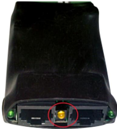
6. Insert an Ethernet cable into any Ethernet port of a device, plug it to a switch or directly to a network card of a computer;
