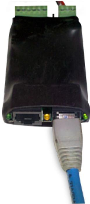
8. A default IP-address of a device is 192.168.0.100. To perform the initial configuration of a device make sure that the address of your computer is in the same IP sub network with a device address. For example, the address of a computer may be: 192.168.0.11 mask: 255.255.255.0.;
